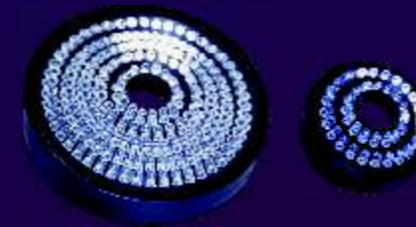
Surface Ring Light Enhance Difficult-to-See Edges Directional Light from 27° to 75° Macro: 5 Rings, 8 Sectors, 40 Segments Standard: 2 Rings, 8 Sectors, 16 Segments Long and Short Working Distances
