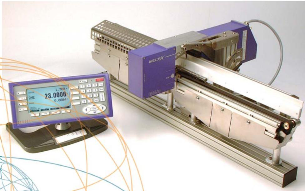
The Grindline.X Laser System has been specially designed for on-line gauging of the outside diameter of products manufactured by through-feed centreless grinding machines, like pins, shock absorbers rods, steering racks or any other part having one ground diameter only to be checked.
